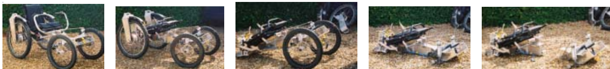
1.Seat back and handlebars collapse. 2. Rear wheel carriers are removed. 3. Front wheels are removed. 4.Frame splits
